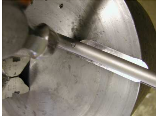
Peen pin to fill hole champher
