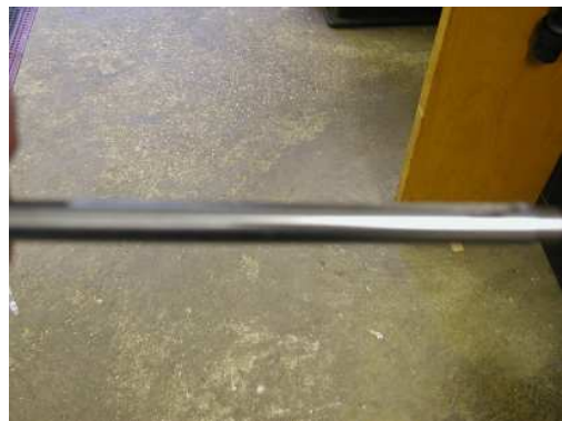
Polish excess pin till smooth to spindle.
