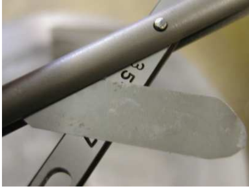
Place shim between leg and spindle on each side of pin.
