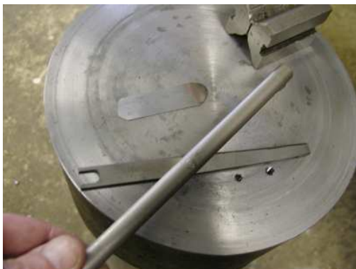
Remove Shim and test that the leg moves freely.
