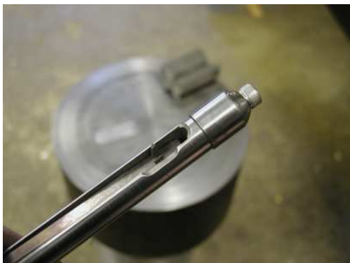
Insert toolbit and pilot.
