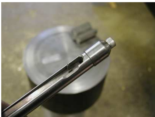
Insert toolbit and pilot.
