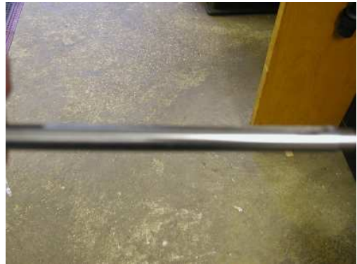
Polish excess pin till smooth to spindle.
