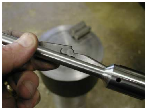
Add shaft leg and test that the leg moves freely.
