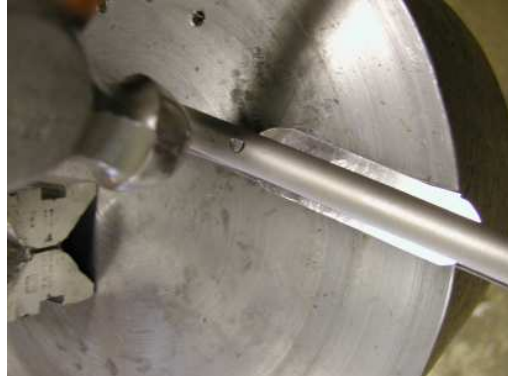
Peen pin to fill hole champher
